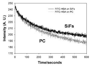
**Fig. 6.** Emission intensity vs. time of FITC-HSA on both silvered and unsilvered modified PC with constant 470 nm excitation, *Top*, and with the laser power adjusted to give the same initial steady state fluorescence intensity, *Bottom*.
