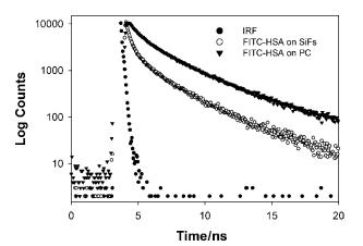
**Fig. 5.** Intensity decays of FITC-HSA on silvered and unsilvered modified PC. The instrumental response function, IRF, is also shown.
